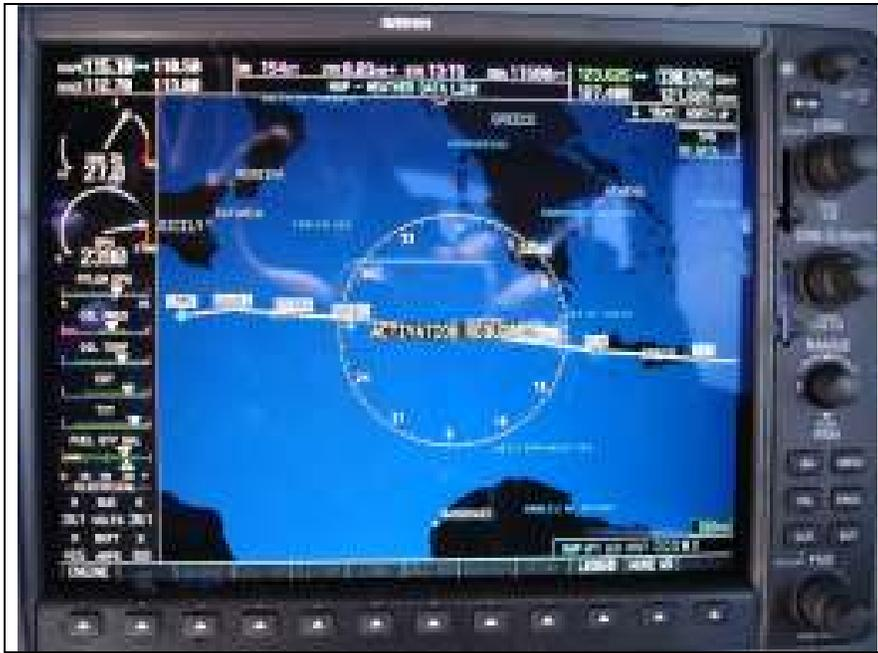
Right Hand screen, showing the programmed routing, and attempting to show real-time weather (but not enabled)
