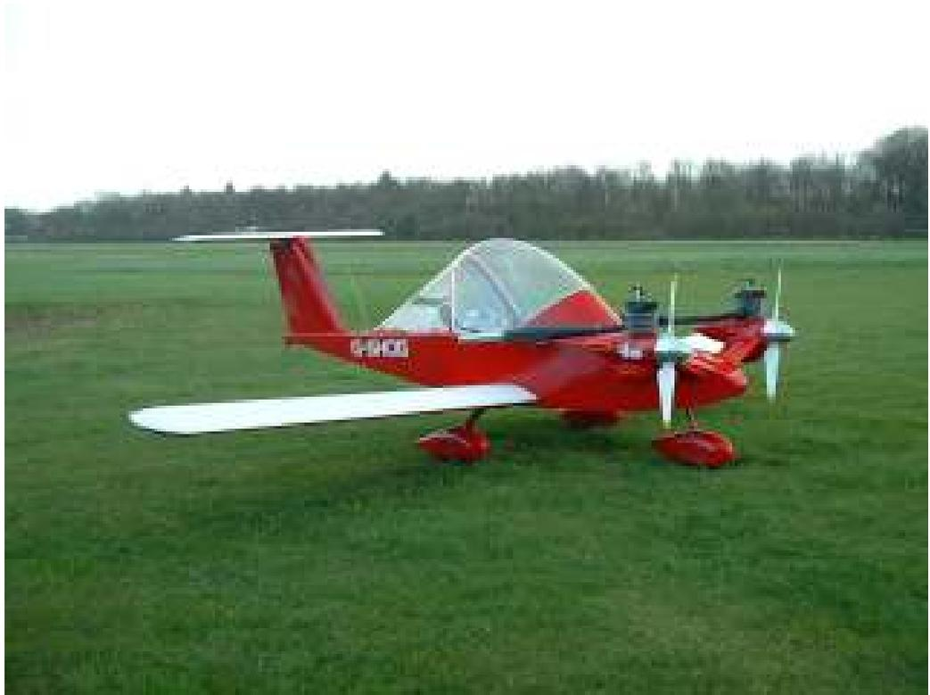
Stalls, power off, come at 57mph with no flap (full width flaperons), 51mph with take-off flap, and 45mph with landing flap. The best recommended single engine speed is 75mph so I am using this for final approach even
