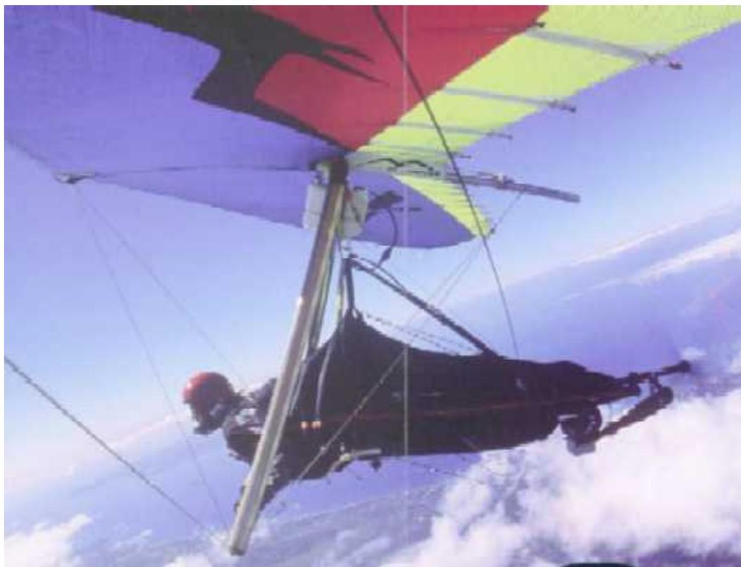
The Mosquito and the Doodle Bug are powered hang gliders. You can lie flat (Mosquito) and be powered by a chain saw engine of 120cc, or you can sit normally with your feet in a stirrup in the Doodle Bug.
